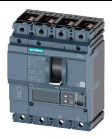
CIRCUIT BREAKER 3VA2 IEC FRAME 100 BREAKING CAPACITY CLASS M ICU=55KA @ 415 V 4POLE, LINE PROTECTION ETU560, LSIG, IN=25A OVERLOAD PROTECTION IR=10A ...25A SHORT CIRCUIT PROTECTION ISD=0,6..10X IN, II=1,5..12X IN NEUTRAL PROTECTION ADJUSTABLE (OFF, UPTO 160%) GROUNDFAULT, SWITCHABLE IG=0,2... 1 X IN, TG=0,050,8MS BUSBAR CONNECTION
