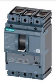
CIRCUIT BREAKER 3VA2 IEC FRAME 160 BREAKING CAPACITY CLASS H ICU=85KA @ 415 V 3POLE, LINE PROTECTION ETU330, LIG, IN=25A OVERLOAD PROTECTION IR=10A ...25A SHORT CIRCUIT PROTECTION II=1,5...12 X IN GROUNDFAULTPROTECTION IG=0,2... 1 X IN, TG=0,1/0,3MS CABLE CONNECTION
