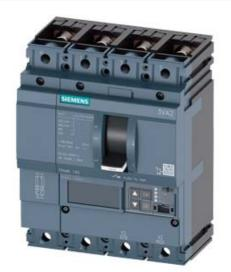
CIRCUIT BREAKER 3VA2 IEC FRAME 160 BREAKING CAPACITY CLASS H ICU=85KA @ 415 V 4POLE, LINE PROTECTION ETU860, LSIG, IN=40A OVERLOAD PROTECTION IR=16A ...40A SHORT CIRCUIT PROTECTION ISD=0,6..10X IN, II=1,5..12X IN NEUTRAL PROTECTION ADJUSTABLE (OFF, UPTO 160%) GROUNDFAULT, SWITCHABLE IG=0,2... 1 X IN, TG=0,050,8MS BUSBAR CONNECTION
