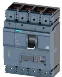
CIRCUIT BREAKER 3VA2 IEC FRAME 630 BREAKING CAPACITY CLASS C ICU=110KA @ 415 V 4-POLE, LINE PROTECTION ETU560, LSIG, IN=500A OVERLOAD PROTECTION IR=200A ...500A SHORT CIRCUIT PROTECTION ISD=0,6..10X IN, II=1,5..14X IN NEUTRAL PROTECTION ADJUSTABLE (OFF, UPTO 100%) GROUND-FAULT, SWITCHABLE IG=0,2... 1 X IN, TG=0,05-0,8MS BUSBAR CONNECTION
