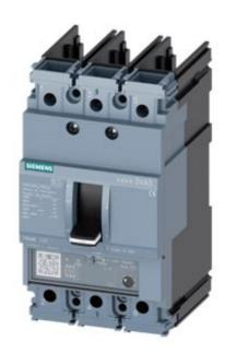
CIRCUIT BREAKER 3VA5 UL FRAME 125 BREAKING CAPACITY CLASS H 65KA @ 480 V 3-POLE, LINE PROTECTION TM230, FTAM, IN=15A OVERLOAD PROTECTION IR=15A FIXED SHORT CIRCUIT PROTECTION II=5...10 X IN UL489 SB (NAVAL), 50 DEG CEL. W/O CONNECTION
