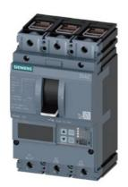
circuit breaker 3VA2 IEC frame 160 breaking capacity class E Icu=200 kA @ 415 V 3-pole, line protection ETU860, LSIG, In=25A overload protection Ir=10A ... 25A short circuit protection Isd=0,6...10xIn, Ii=1,5...12xIn cable connection
