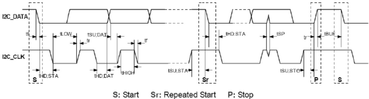
Figure 2 I<sup>2</sup>C Timing Diagram
