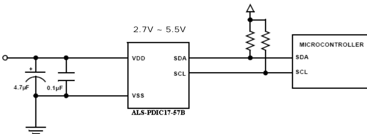
Figure 17 Application Circuit
