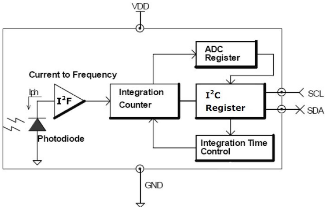
Figure 1 ALS-PDIC17-57B/TR8 Functional Block Diagram
