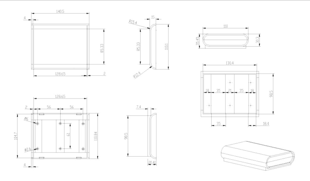
The case has 4 screws 2.9x6.5 (DIN7981)
