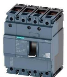
CIRCUIT BREAKER 3VA1 IEC FRAME 160 BREAKING CAPACITY CLASS H ICU=70KA @ 415 V 4-POLE, LINE PROTECTION TM210, FTFM, IN=100A OVERLOAD PROTECTION IR=100A FIXED SHORT CIRCUIT PROTECTION II=10 X IN NEUTRAL PROTECTION 50% BUSBAR CONNECTION
