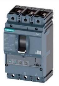
CIRCUIT BREAKER 3VA2 IEC FRAME 250 BREAKING CAPACITY CLASS L ICU=150KA @ 415 V 3POLE, LINE PROTECTION ETU350, LSI, IN=250A OVERLOAD PROTECTION IR=100A ...250A SHORT CIRCUIT PROTECTION ISD=1,5... 10 X IR, II=10 X IN BUSBAR CONNECTION
