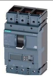
CIRCUIT BREAKER 3VA2 IEC FRAME 400 BREAKING CAPACITY CLASS M ICU=55KA @ 415 V 3-POLE, LINE PROTECTION ETU550, LSI, IN=400A OVERLOAD PROTECTION IR=160A ...400A SHORT CIRCUIT PROTECTION ISD=0,6..10X IN, II=1,5..10X IN NEUTRAL PROTECTION OPTIONAL WITH EXT. CT;UPTO 160% BUSBAR CONNECTION
