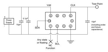
Figure 12. LVCMOS Test Circuit (I<sup>2</sup>C Control)
