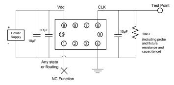
Figure 11. Clipped Sinewave Test Circuit (NC Function)
