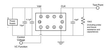
Figure 9. Clipped Sinewave Test Circuit (VC Function)
