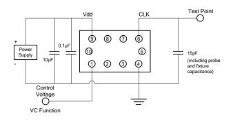
Figure 8. LVCMOS Test Circuit (VC Function)
