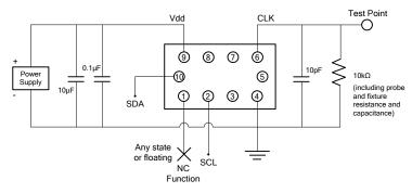
Figure 13. Clipped Sinewave Test Circuit (I<sup>2</sup>C Control)
