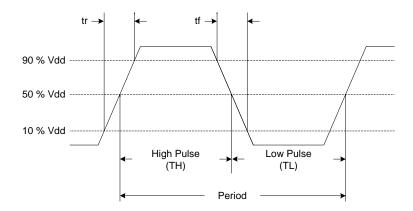
Figure 14. LVCMOS Waveform Diagram
