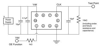
Figure 6. LVCMOS Test Circuit (OE Function)
