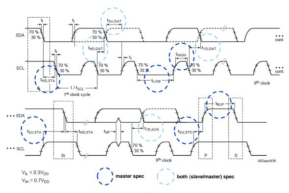
Figure 35. I<sup>2</sup>C Timing Diagram
