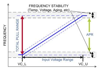
Figure 26. Typical SiTime VCTCXO FV Characteristic
