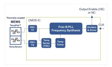
Figure 20. Block Diagram - TCXO
