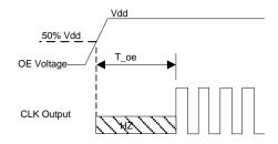
T\_oe: Time to re-enable the clock output
