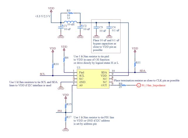
Figure 36. Schematic Example - DCTCXO
