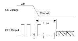
T\_oe: Time to put the output in High Z mode
