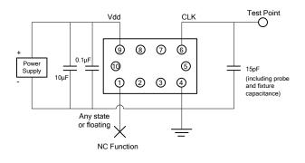
Figure 10. LVCMOS Test Circuit (NC Function)
