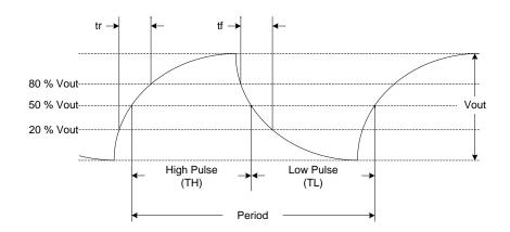
Figure 15. Clipped Sinewave Waveform Diagram
