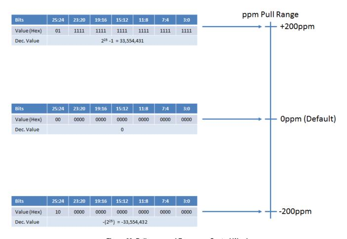
Figure 29. Pull range and Frequency Control Word
