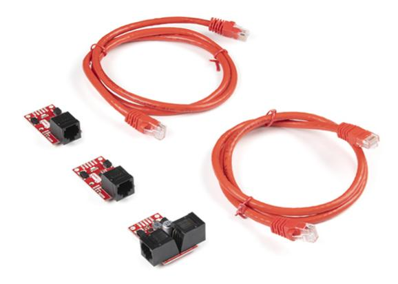
The SparkFun QwiicBus Kit comes with everything you need to get started with the SparkFun QwiicBus system in one handy package. The kit includes two QwiicBus EndPoints, one MidPoint and two 3ft Ethernet cables.
