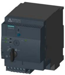
SIRIUS, COMPACT STARTER, REVERSING STARTER 690 V, 24 V AC/DC, 50 ... 60 HZ, 1 ... 4 A, IP20, MAIN CIRCUIT CONNECTION: PLUG-IN, W/O TERMINALS, AUXILIARY CIRCUIT CONNECTION: SCREW TERMINAL
