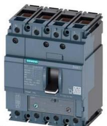
CIRCUIT BREAKER 3VA1 IEC FRAME 160 BREAKING CAPACITY CLASS S ICU=36KA @ 415 V 4-POLE, LINE PROTECTION TM240, ATAM, IN=80A OVERLOAD PROTECTION IR=56A ...80A SHORT CIRCUIT PROTECTION II=5...10 X IN NEUTRAL UNPROTECTED CABLE CONNECTION
