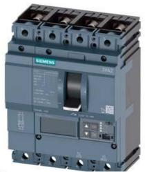
CIRCUIT BREAKER 3VA2 IEC FRAME 100 BREAKING CAPACITY CLASS L ICU=150KA @ 415 V 4POLE, LINE PROTECTION ETU850, LSI, IN=100A OVERLOAD PROTECTION IR=40A ...100A SHORT CIRCUIT PROTECTION ISD=0,6..10X IN, II=1,5..12X IN NEUTRAL PROTECTION ADJUSTABLE (OFF, UPTO 100%) BUSBAR CONNECTION
