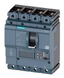
CIRCUIT BREAKER 3VA2 IEC FRAME 160 BREAKING CAPACITY CLASS M ICU=55KA @ 415 V 4POLE, LINE PROTECTION ETU850, LSI, IN=100A OVERLOAD PROTECTION IR=40A ...100A SHORT CIRCUIT PROTECTION ISD=0,6..10X IN, II=1,5..12X IN NEUTRAL PROTECTION ADJUSTABLE (OFF, UPTO 160%) BUSBAR CONNECTION
