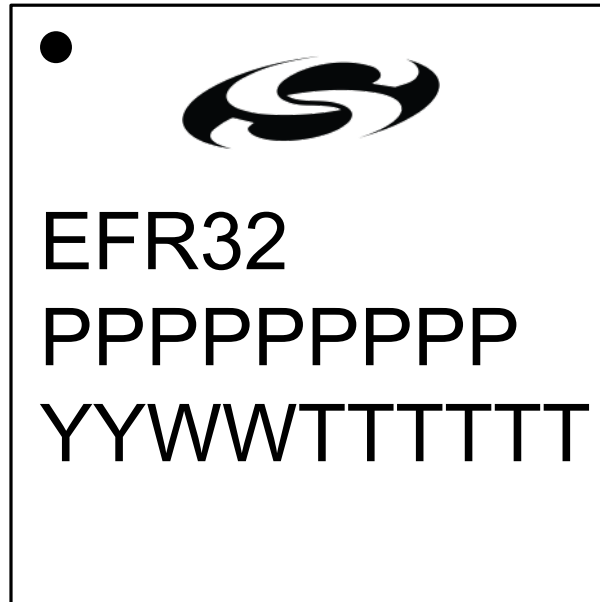
Figure 8.3. QFN32 Package Marking
