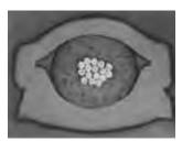
**Insulation Crimp Cross Section**
