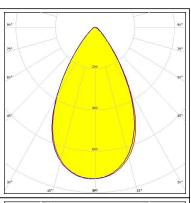
LED LC010C G2 **FWHM** 45.0° 82 % Efficiency 1.200 cd/lm Peak intensity
