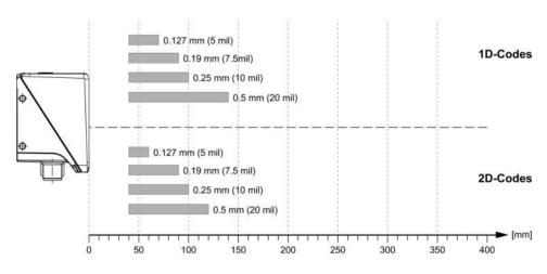
Part no.: 50128788 – DCR 202i FIX-N1-102-R3-P – Stationary 2D-code reader
