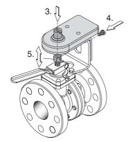
6. Install the actuator (puck) on top of the shaft and the valve sensor on the sensor plate.
