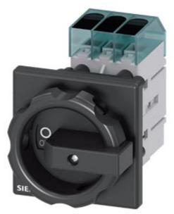
Switch disconnector 3LD3, main switch 3-polig, lu 32A operational switch at AC-23 A at 400 V 11,5 kW front mounted Base mounting with center-hole 22,5 mm rotary operationg mechanism black 66 x66 mm
