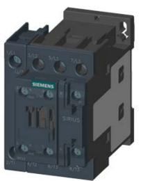
4NO CONTACTOR, AC1: 50A AC 230V 50HZ 4-POLE, 4NO, SZ: S0, SCREW TERMINAL 1NO+1NC INTEGR.
