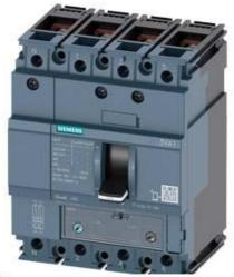
CIRCUIT BREAKER 3VA1 IEC FRAME 160 BREAKING CAPACITY CLASS S ICU=36KA @ 415 V 4-POLE, LINE PROTECTION TM240, ATAM, IN=63A OVERLOAD PROTECTION IR=44,1A ...63A SHORT CIRCUIT PROTECTION II=5 X IN NEUTRAL PROTECTION 100% BUSBAR CONNECTION
