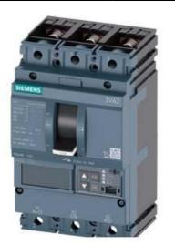
CIRCUIT BREAKER 3VA2 IEC FRAME 100 BREAKING CAPACITY CLASS L ICU=150KA @ 415 V 3POLE, LINE PROTECTION ETU860, LSIG, IN=25A OVERLOAD PROTECTION IR=10A ...25A SHORT CIRCUIT PROTECTION ISD=0,6..10X IN, II=1,5..12X IN NEUTRAL PROTECTION OPTIONAL WITH EXT. CT,UPTO 160% GROUNDFAULT, SWITCHABLE IG=0,2... 1 X IN, TG=0,050,8MS BUSBAR CONNECTION
