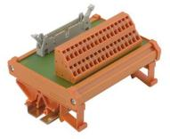
Passive interface for 10 ... 64 signals for adapting preassembled leads with plug connectors to IEC 603-1 / DIN 41651 to screw or tension clamp connection systems.
