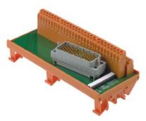
Weidmuller's passive interface units are used for adapting hermaphrodite ELCO multi-pole connectors, for input and output, to screw terminal systems. The hermaphrodite contact is a fork-type contact that is identical in design on both sides of the connection, but with one fork turned through 90° to engage with the other.
