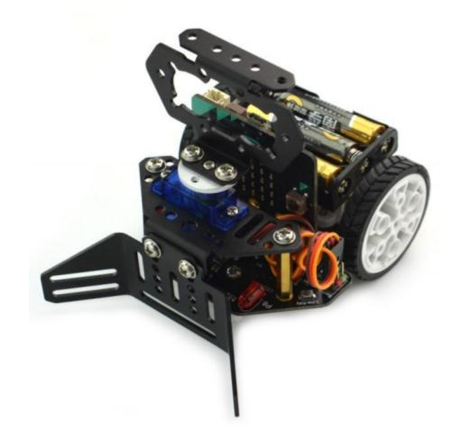
micro: Maqueen with micro:Maqueen Mechanic-Push **FEATURES** Support for Maqueen 4.0 and later Support for Maqueen Plus Metal gear servo, reliable quality Metal servo connection plate for easy installation 0 ~ 180 deg control angle Aluminum alloy material, sandblasting oxidation process, excellent quality. **SPECIFICATION** Servo Weight: 12g ± 1g
