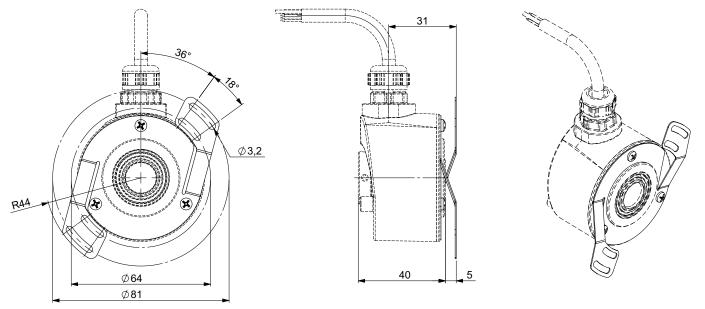
DH05S14/OM/ Flange side clamping, Connection IPR (Radial M23)", coupling 9445/016 mounted on the body
