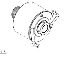
DH05\_14 Standard clamping, Connection G3R (Radial Cable), coupling 9445/012 mounted on the body
