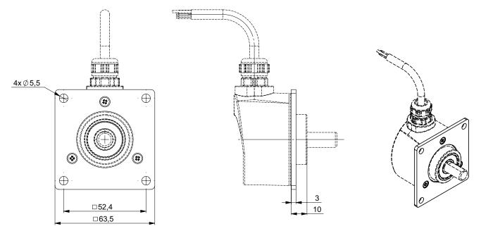
DHK5\_14 Connection I6A (Axial M23), coupling 9445/016 mounted on the body
