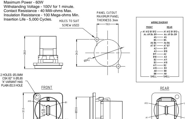
N.B. FUNCTIONALITY IS AFFECTED BY CABLE QUALITY, LENGTH AND CABLE WIRING CONFIGURATION. NOT COMPATIBLE FOR POWER DELIVERY (PD) CHARGING.
