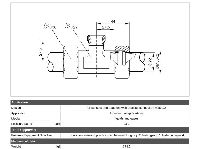
Recommendation: precision steel pipes 22 x 1,5 DIN 2391/ISO 3304 brass (2.0401)
