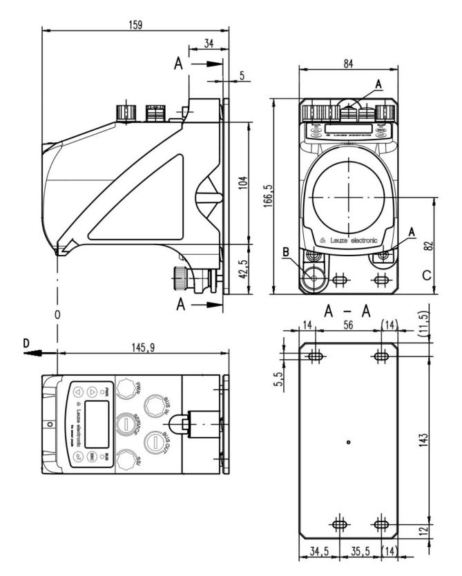
A M 5 screw for alignment
