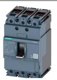
CIRCUIT BREAKER 3VA1 IEC FRAME 100 BREAKING CAPACITY CLASS N ICU=25KA @ 415 V 3-POLE, LINE PROTECTION TM210, FTFM, IN=16A OVERLOAD PROTECTION IR=16A FIXED SHORT CIRCUIT PROTECTION II=10 X IN CABLE CONNECTION
