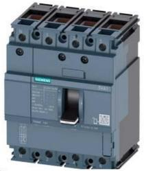
CIRCUIT BREAKER 3VA1 IEC FRAME 160 BREAKING CAPACITY CLASS S ICU=36KA @ 415 V 4-POLE, LINE PROTECTION TM210, FTFM, IN=100A OVERLOAD PROTECTION IR=100A FIXED SHORT CIRCUIT PROTECTION II=10 X IN NEUTRAL UNPROTECTED CABLE CONNECTION
