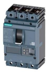
CIRCUIT BREAKER 3VA2 IEC FRAME 160 BREAKING CAPACITY CLASS C ICU=110KA @ 415 V 3POLE, LINE PROTECTION ETU560, LSIG, IN=25A OVERLOAD PROTECTION IR=10A ...25A SHORT CIRCUIT PROTECTION ISD=0,6..10X IN, II=1,5..12X IN NEUTRAL PROTECTION OPTIONAL WITH EXT. CT,UPTO 160% GROUNDFAULT, SWITCHABLE IG=0,2... 1 X IN, TG=0,050,8MS BUSBAR CONNECTION
