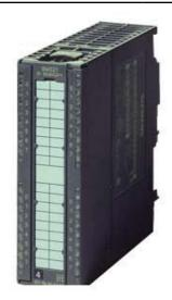
SIPLUS S7-300 SM321 16DE 0-1 LEVEL AT ABOUT 11.2V WITH CONFORMAL COATING BASED ON 6ES7321-7BH01-0AB0 . DIGITAL INPUT SM 321, GALVANICALLY ISOLATED, 16 DI, DC 24V, 1 X 20 PIN, PROCESS INTERRUPT, DIAGNOSTICS, FIT FOR ISOCHRONE MODE
