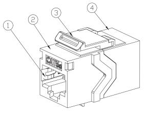
ELECTRICAL CURRENT RATING : 1.5A DIELECTRIC WITHSTANDING VOLTAGE : 1000VDC INSULATION RESISTANCE : 500 M $\Omega$  MIN. CONTACT RESISTANCE : 20 m $\Omega$  MAX. MECHANICAL (1) Earthing lug material: Stainless steel SUS304 (2) Front cover: Nickel plated zinc alloy
