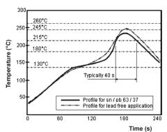
Infrared soldering profile for Chip Resistors
