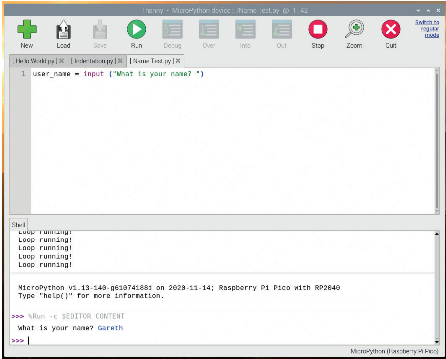
▲ Figure 2-7: The input function lets you ask a user for some text input
