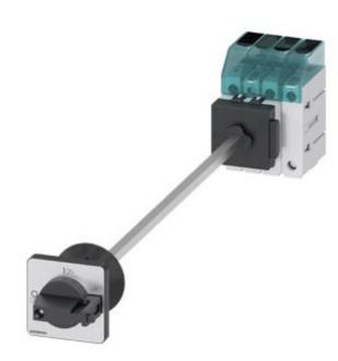
Switch disconnector 3LD3, main switch 3-polig + N, lu 63A operational switch at AC-23 A at 400 V 22,0 kW floor mounting Base mounting with door coupling center-hole 22,5 mm knob-operated mechanism black 48 x 48 mm
