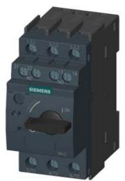
CIRCUIT-BREAKER SZ S00, FOR TRANSFORMER PROT. A-RELEASE 0.22...0.32A, N-RELEASE6.5A SCREW CONNECTION, STANDARD SW. CAPACITY W. TRANSVERSE AUX. SWITCH 1NO+1NC
