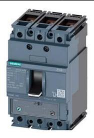
CIRCUIT BREAKER 3VA1 IEC FRAME 160 BREAKING CAPACITY CLASS S ICU=36KA @ 415 V 3-POLE, LINE PROTECTION TM240, ATAM, IN=40A OVERLOAD PROTECTION IR=28A ...40A SHORT CIRCUIT PROTECTION II=5...10 X IN BUSBAR CONNECTION
