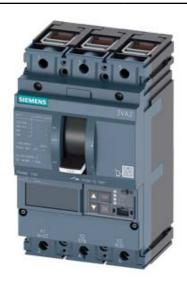
CIRCUIT BREAKER 3VA2 IEC FRAME 100 BREAKING CAPACITY CLASS H ICU=85KA @ 415 V 3POLE, LINE PROTECTION ETU560, LSIG, IN=40A OVERLOAD PROTECTION IR=16A ...40A SHORT CIRCUIT PROTECTION ISD=0,6..10X IN, II=1,5...12X IN NEUTRAL PROTECTION OPTIONAL WITH EXT. CT,UPTO 160% GROUNDFAULT, SWITCHABLE IG=0,2... 1 X IN, TG=0,050,8MS CABLE CONNECTION
