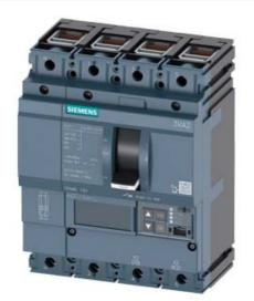
CIRCUIT BREAKER 3VA2 IEC FRAME 160 BREAKING CAPACITY CLASS H ICU=85KA @ 415 V 4POLE, LINE PROTECTION ETU550, LSI, IN=160A OVERLOAD PROTECTION IR=64A ...160A SHORT CIRCUIT PROTECTION ISD=0,6..10X IN, II=1,5..10X IN NEUTRAL PROTECTION ADJUSTABLE (OFF, UPTO 100%) CABLE CONNECTION
