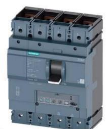
CIRCUIT BREAKER 3VA2 IEC FRAME 400 BREAKING CAPACITY CLASS M ICU=55KA @ 415 V 4-POLE, LINE PROTECTION ETU330, LIG, IN=400A OVERLOAD PROTECTION IR=160A ...400A SHORT CIRCUIT PROTECTION II=1,5...10 X IN NEUTRAL PROTECTION ADJUSTABLE(OFF,50%,100%) GROUND-FAULT-PROTECTION IG=0,2... 1 X IN, TG=0,1/0,3MS BUSBAR CONNECTION
