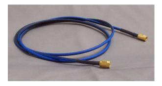
The 110A probe cable is designed to connect the 100 series probes to the 150A amplifier or other instruments. This double-shielded cable has good RF performance from DC to 6 GHz.
