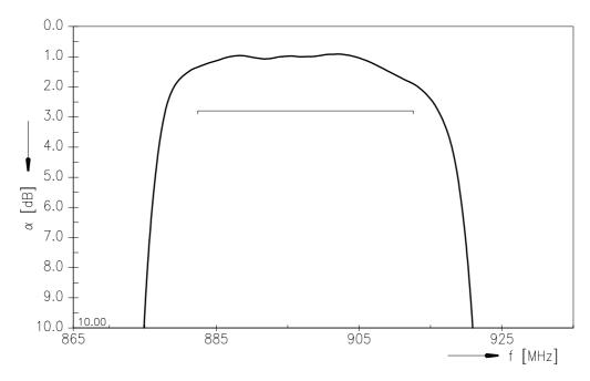
Frequency Response TX-ANT (Passband, CW test signal)
