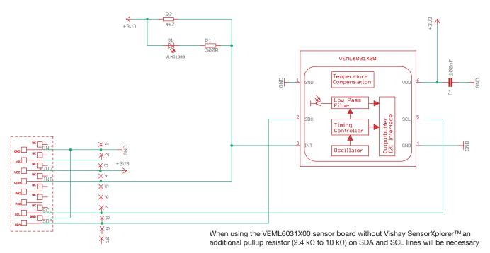
Fig. 4 - Schematic of the Schematic of the VEML6031X00 Sensor Board
