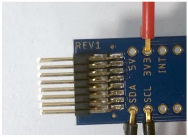
Fig. 3 - Connection of the Sensor Board (power supply and I<sup>2</sup>C lines)
