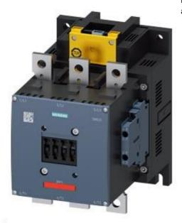
Contactor AC3: 110kW / 400 V 3-pole Size S10 Coil AC 50/60Hz and DC 96...127 V x (0,8...1,1) auxiliary contacts: 2 NO + 2 NC permanently mounted (SUVA) Main: busbar connections coil and auxilliary: screw terminal
