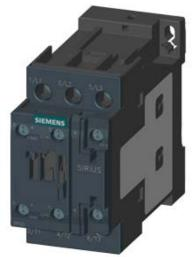
CONTACTOR, AC-3, 7.5KW/400V, 1NO+1NC, DC 48V, 3-POLE, SZ S0 SCREW TERMINAL
